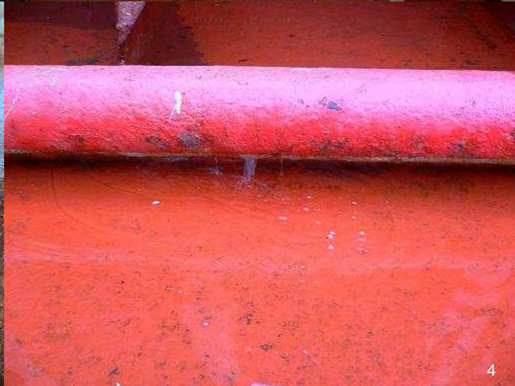
MV Universal Challenger: Poor working and living conditions (1, 2), bulkhead corrosion (3), leaking main fire line (4)
