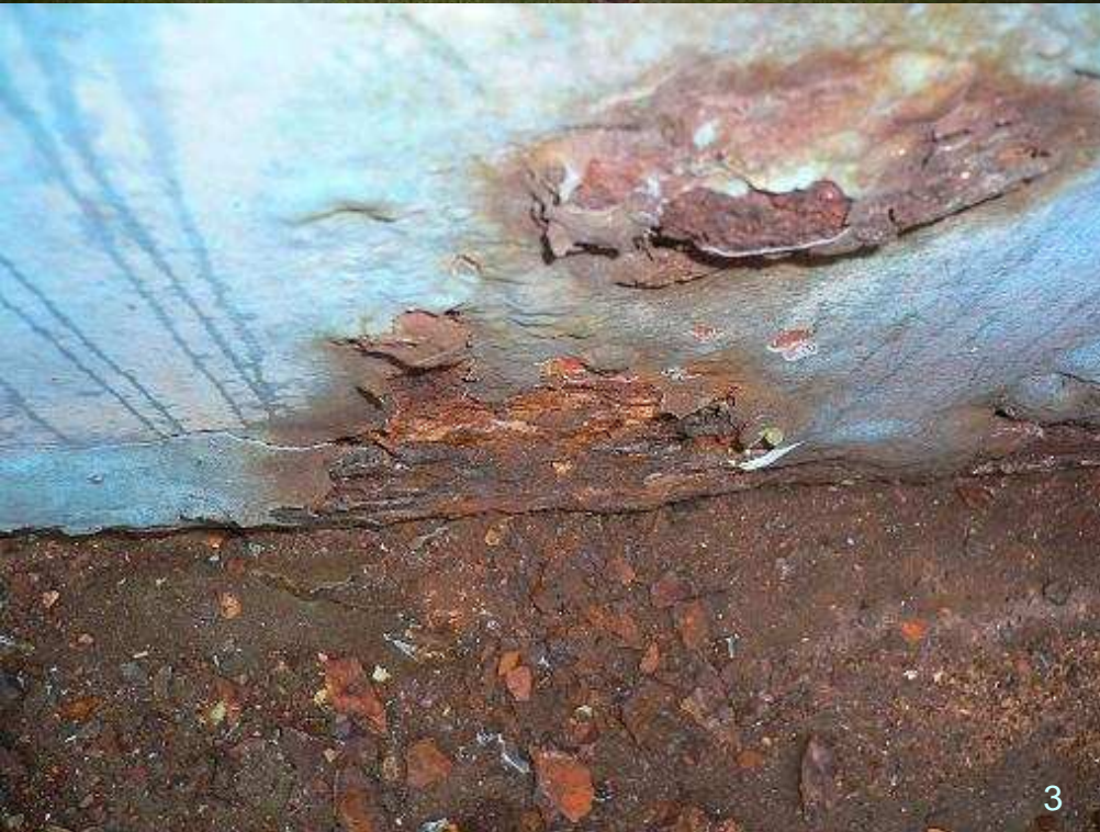
MV Universal Challenger: Poor working and living conditions (1, 2), bulkhead corrosion (3), leaking main fire line (4)
